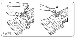
Pull bulb out of socket. Do NOT twist. Gently push bulb into socket to replace.
